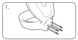
Insert the M8 Hex Bolts through the Orbis fixing holes.
