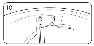
Secure in position with M8 Washers and Nuts using 13mm Spanners.
