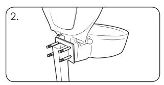
Insert the Orbis with the bolts through the holes of the Orbis Post(supplied separately).
