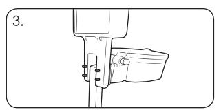
Locate the Sign Carrier's fixing holes on to the exposed bolts protruding through the rear of the Orbis Post.
