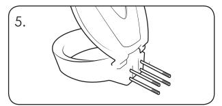
Insert the M8 Hex Bolts through the Orbis fixing holes.
