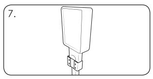
Then align the Sign Carrier fixing holes with the 2 Point Bracket and the Orbis Post.
