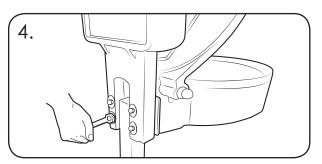
Secure in position with M8 Washers and Nuts using 13mm Spanners.
