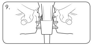
Locate second Orbis onto the exposed fixing bolts, which will hold all the units together.
